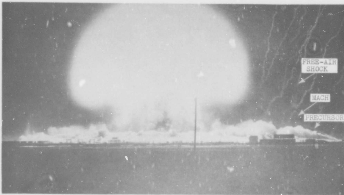
Figure 3.43 Shot 12, Photograph of Shock Along Asphalt 1,430 ft from Ground Zero at t = 0.213 sec (Film 28381).
